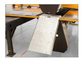
Frontal reclining table for unloading the workpieces
