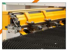
Automatic and programmable sheet metal locking clamps
